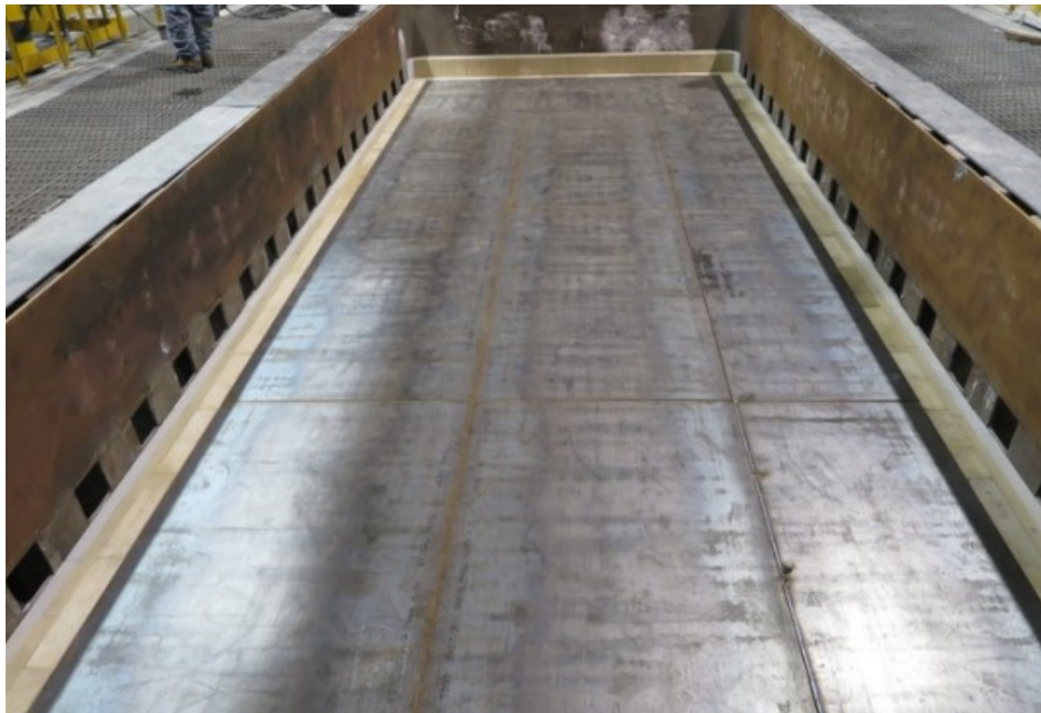
Figure 7. Cell construction using steel plate
